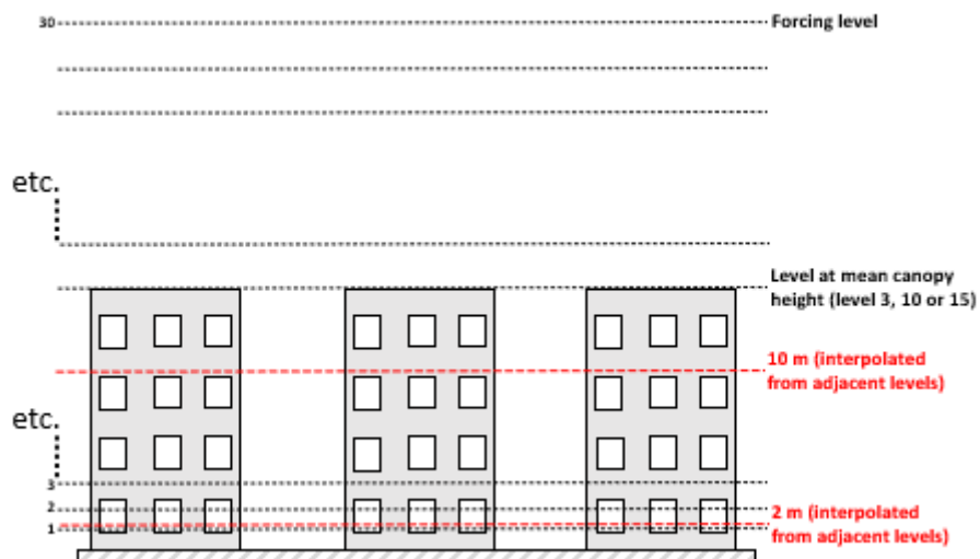
Fig. 7.6: SUEWS-RSL module assumes the RSL has 30 layers that are spread between the canopy and within the atmosphere above
